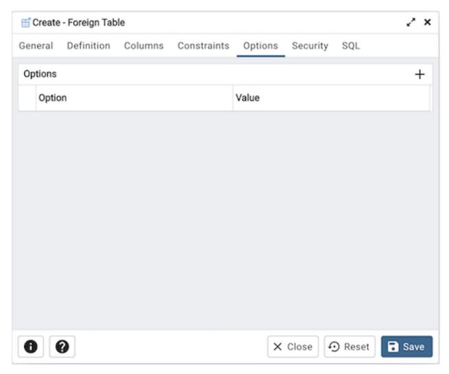
Use the fields in the *Options* tab to specify options to be associated with the new foreign table or one of its columns; the accepted option names and values are specific to the foreign data wrapper associated with the foreign server. Click the *Add* icon (+) to add an option/value pair.
