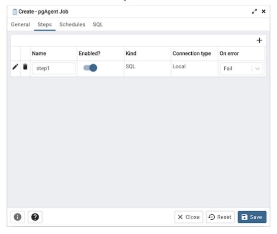
Use the *Steps* tab to define and manage the steps that the job will perform. Click the Add icon (+) to add a new step; then click the compose icon (located at the left side of the header) to open the step definition dialog:
