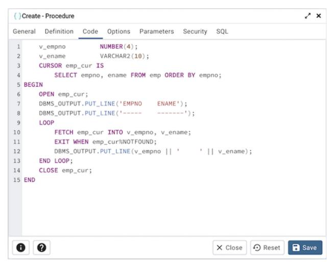
• Use the *Code* field to specify the code that will execute when the procedure is called.
