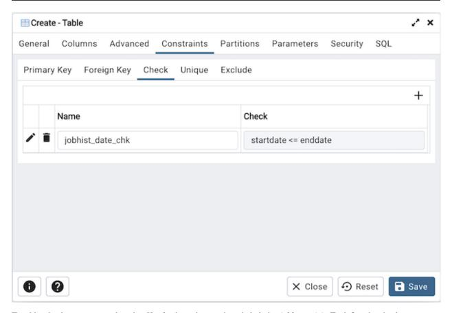
To add a check constraint, select the *Check* tab on the panel, and click the *Add* icon (+). To define the check constraint, click the *Edit* icon to the left of the *Trash* icon. A dialog similar to the *Check* dialog (accessed by right clicking on *Constraints* in the pgAdmin tree control) opens.
