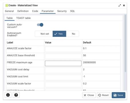
Use the tabs nested inside the *Parameter* tab to specify VACUUM and ANALYZE thresholds; use the *Table* tab and the *Toast Table* tab to customize values for the table and the associated toast table. To change the default values:
