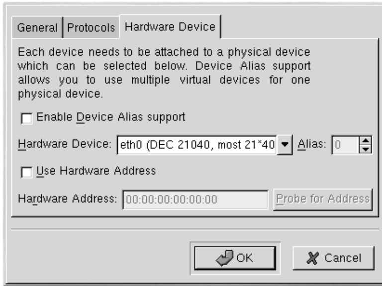
Figure 6–2 Adding an Ethernet Device
